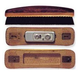
With its small size and close-focusing lens (the better to copy documents with), the Minox camera was popular in espionage circles and hidden in a variety of concealment devices, like this gentleman's clothing brush. The two halves of the brush discreetly locked together and could only be unfastened by inserting a pin into a camouflaged hole.
